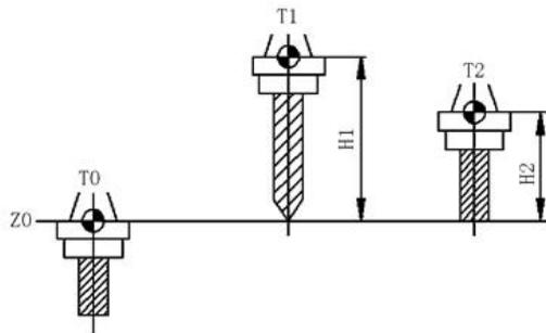
Figure 2-30 Length compensation principle
