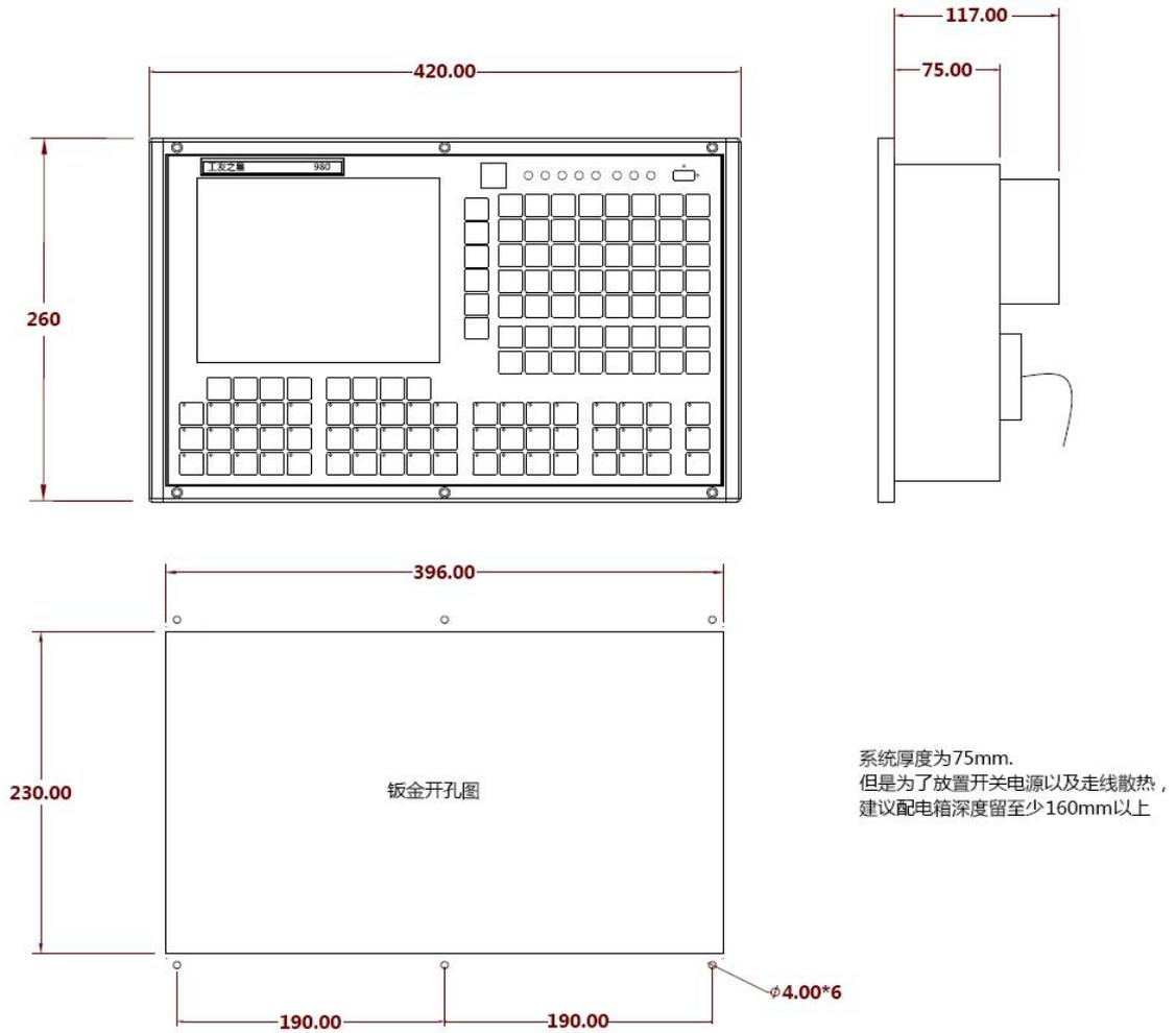
Figure 4-1 Installation dimensions of the system
