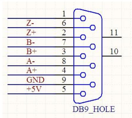
Figure 4-17 Spindle encoder interface
