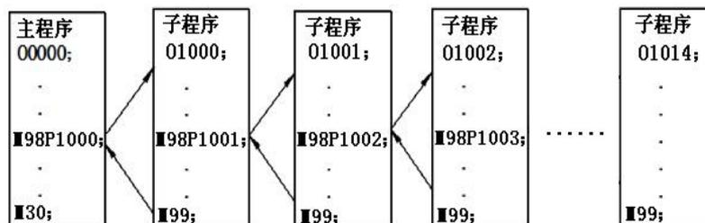
If M99 is executed in the main program, the control returns to the beginning of the main program and the main program is executed from scratch.
