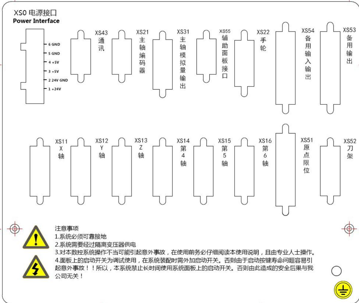
Figure 4-2 Back view of the interface layout
