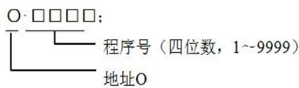
The program starts with the program number and ends with M30 or M99. The basic program segment structure is shown in Table 2-4:
