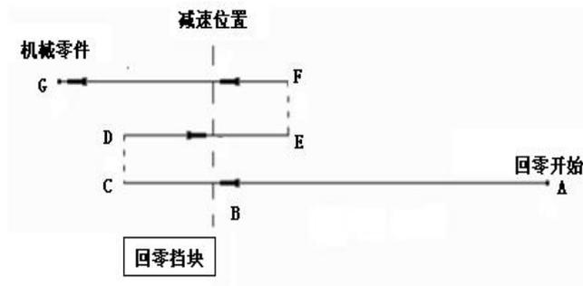
Figure 3-45 Schematic diagram of the reference reference point process
