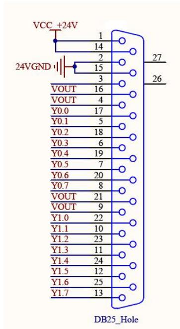
Figure 4-12 The standby output interface
