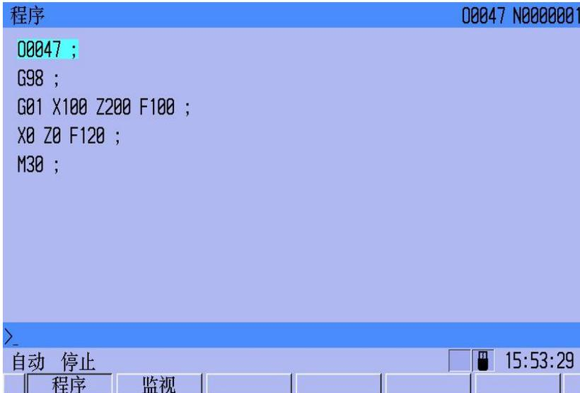
Figure 3-16 Display interface for program execution
