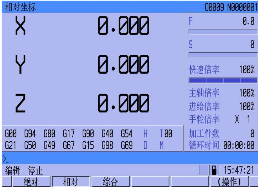
Figure 3-9 The relative coordinate interface
