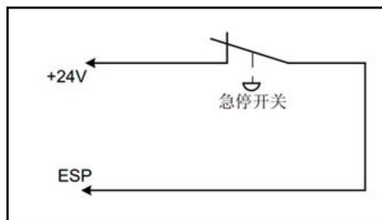
Figure 3-5 Normally closed emergency stop signal circuit connection
