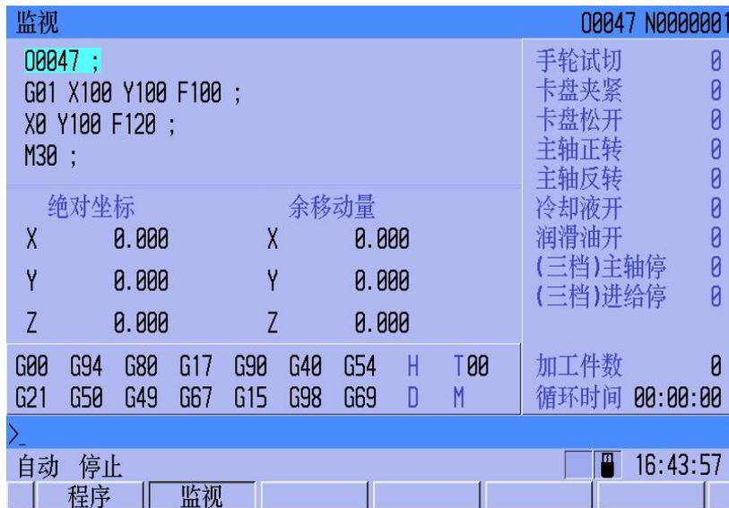
Figure 3-17, the program monitor PLC signal customization interface
