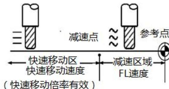
Figure 3-6 Schematic diagram of the process back to the reference point
