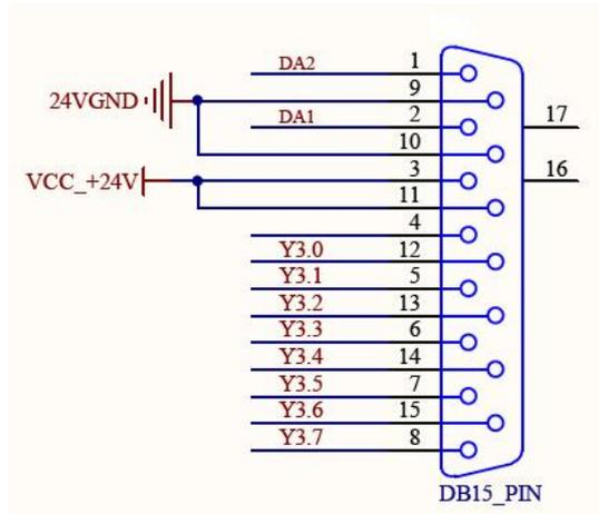
Figure 4-11, the spindle interface
