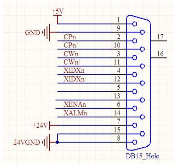
Figure 4-3 Feed motor interface
