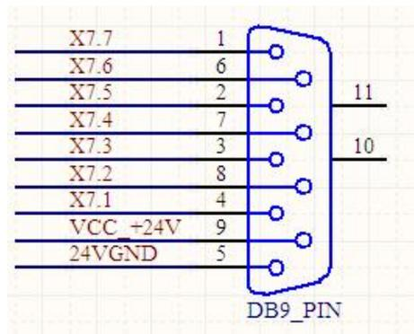
Figure 4-20 Auxiliary panel interface
