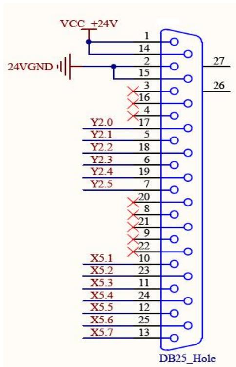
Figure 4-13 Alternate input / output interface
